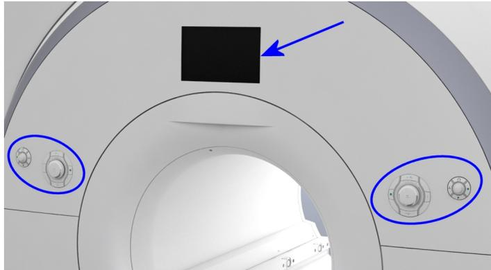
**Control units** The control units are located at the right and the left side of the patient table at the front of the magnet cover. Optionally, additional control units are located at the back of the magnet.
