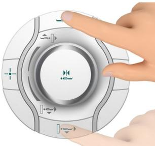
2 To reset the table stop, turn the **Table Stop** button clockwise until it releases mechanically. Then simultaneously press the **Table Up/Inward** and the **Table Down/Outward** button fully.
