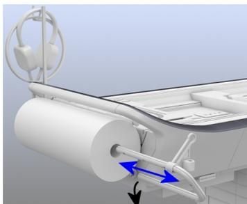
The paper roll holder can be mounted at the foot end of the table below the handle. It includes a holder to reposit the headphones and can be removed if required. To replace the paper roll (disposable), you need to detach the headphone holder. If you remove the stick on the paper roll, you can pull out the right mounting bracket. Then you can replace the roll and let the bracket again lock into place.
