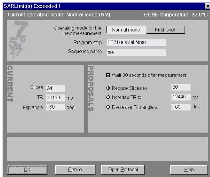
This dialog window includes suggested changes to the examination parameters which allow the examination to continue. In addition, a button in the dialog window may be used to change the operating mode.
